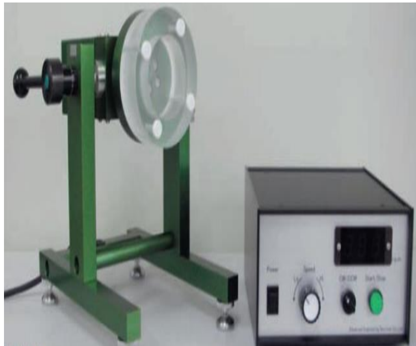
Fig 2: The uniaxial (2-D) Clinostat (in horizontal position) and its control box. Image Source – Credit: Microgravity-Simulation Laboratory, Engineering and Space Systems Department (ESS), National Space Research and Development Agency (NASRDA), Abuja, Nigeria
